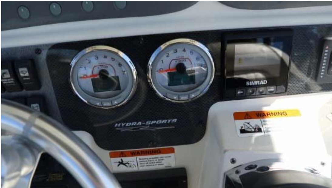
The new panel has a pair of digital gauges that are more accurate and easier to read as well as a Simrad display for selectable engine parameters.
