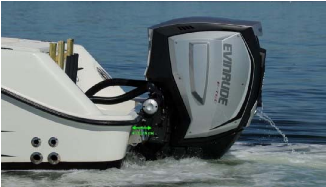
The new engines are offset 4" (10.16 cm) further back from the transom than the old engines.
