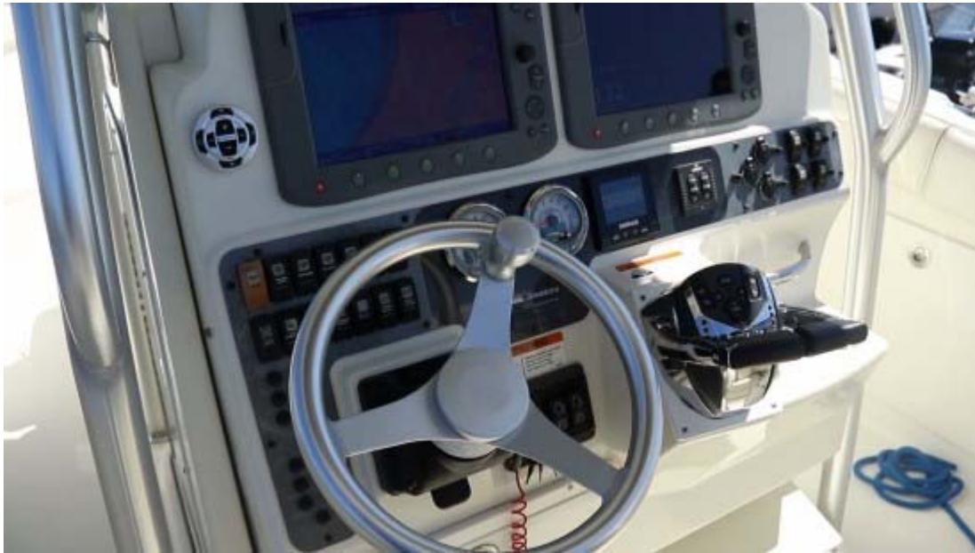
The new controls are easier to use and much more functional than the old. With automatic sync and drive by wire, RPM settings can be exact.
